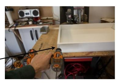
Screw the sides together and screw the sides to the base to form a box using the 2" screws.
