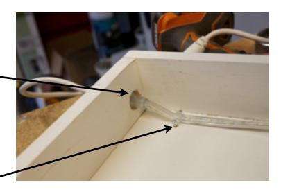
Use the included clamps to mount the light rope to the base. If you run out of the included clamps you can use plastic electrical clamps. Pre-drill the holes for the #6 X 1/2 inch screws.
