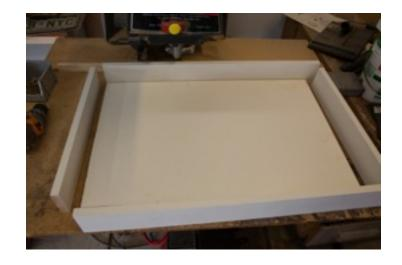
The 18.5 pieces will fit inside both ends of the 29" pieces creating an inner space of 18.5" X 27.75" (a 3 X 2 ratio of the lighted area to match the camera sensor)
