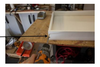
Drill large hole to put the power cable through the side. The size will depend on what kind of cord your lights have.
